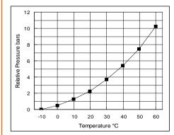
Specific heat (liquid at 0°C):  $0.324 \text{ kcal/kg}^{\circ}C$ Latent heat of vaporisation at 0°C: 91.02 kcal/kgLatent heat of vaporisation at 50°C: 79.71 kcal/kgMelting point (P = 1 atm):  $-72.7^{\circ}C$ Boiling point (P = 1 atm):  $-10.0^{\circ}C$
